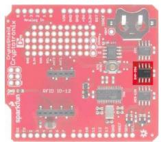
This chip, like the other crypto chips, is *one-time-programmable*. This means that once you run certain commands on the chip, it **can not** be reversed. This is a security feature.
