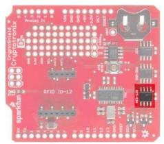
The Atmel AES132 is an AES encrypted EEPROM that can store up to 32Kb of data. Specifically, it uses AES with a 128 bit key in CCM mode.
