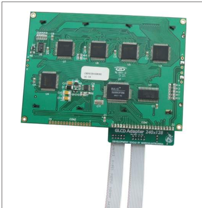
Figure 5: GLCD Adapter additional board connected to a GLCD display
