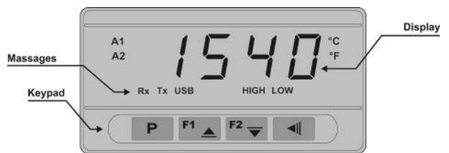
Figure 08 - Identification of the front panel parts
