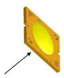
5.0.2 – Apply the M3 or 4-40 screws with 0.2 (MIN) to 0.8 Nm (MAX) of force on each screw TORQUE: CERAMIC 0.20 N-M MIN TO 0.40 N-M MAX;
