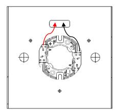
5.0.7 – Pull wires through holes ensuring that the holder is placed and fits flush on the top of the heat sink or with the mounting area on the inside of the fixture
