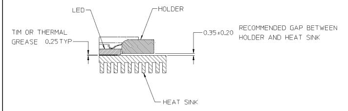
6.0.2 If TIM material exceeds 0.25 mm thickness, the LED holder may tilt excessively when screwed down. It is recommended that the TIM extends to the area below the LED holder as shown below to provide support under the screws.
