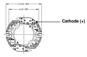
Note: wires can be inserted at either end of the Cathode (+) wire trap
