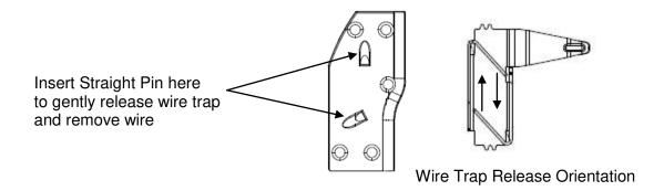
Note: Do not overstress beam when removing, only gentle pressure of 4 Newton or less is required
