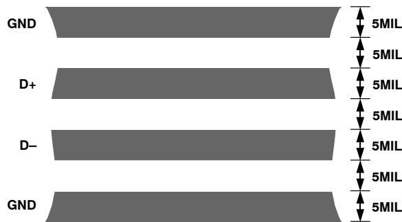
Figure 34. Typical Arrangement of Signal Tracks
