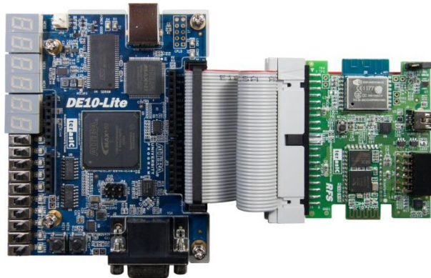
Figure 4-4 Setup ESP8266 Client Demo on DE10-Lite
