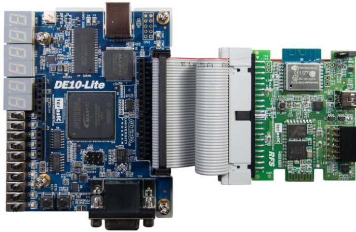
Figure 4-34 Setup Sensor demo on DE10-Lite
