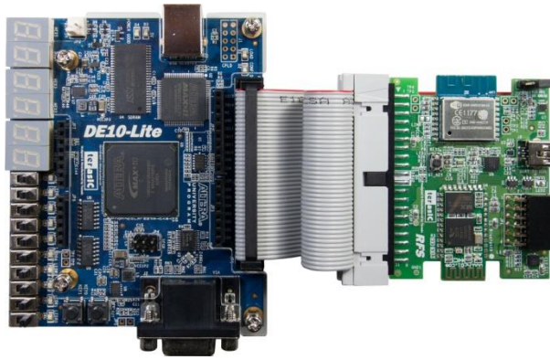
Figure 4-10 Setup ESP8266 Web Server Demo on DE10-Lite
