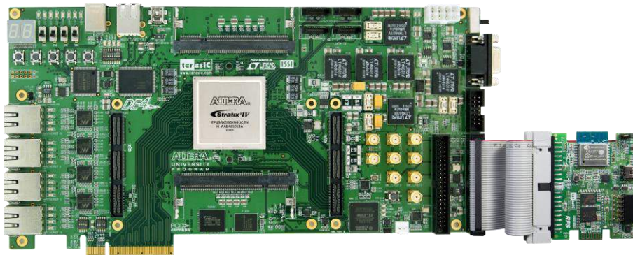
Figure 4-12 Setup ESP8266 Web Server Demo on DE4
