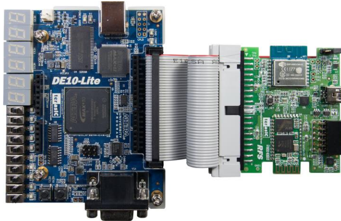
Figure 4-18 Setup HC-05 Configuration Demo to DE10-Lite
