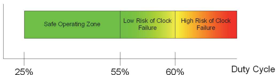
Figure 20.2. Interpreting Oscillation Robustness (Duty Cycle) Test Results
