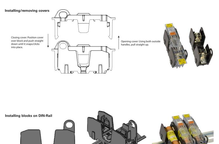
Place one edge of DIN-Rail in fuse block base, then rotate block down until it clicks into place.
