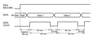
Measurement data is output every 64 ms while the REQUEST signal remains ON.
