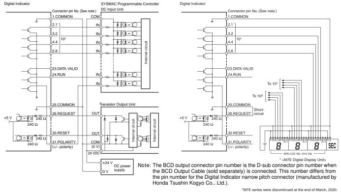
Refer to the following User's Manual for application precautions and other information required when using the Digital Indicator: K3HB-S/-X/-V/-H Digital Indicator User's Manual (Cat. No. N128)
