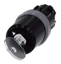
key-operated switch Siemens, 22 mm, round, plastic with metal front ring, lock no. LSG1, with 2 keys, 2 switch positions O-I, latching, actuating angle 90°, 10:30h/13:30h, key removal O+I, with laser labeling, upper case
