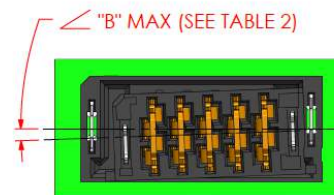
INITIAL Z AXIS ANGULAR MISALIGNMENT
