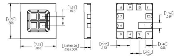
TOLERANCE IS ±.005 [0.13] DIMENSIONS ARE IN INCHES AND [MILLIMETERS]
