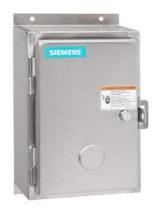
Non-reversing NEMA contactor, Size 1, Three phase full voltage, Contactor amp rating 27A, 3 wire (NO aux included), 110-120/220-240VAC 60Hz coil, Non-combination type, Encl NEMA type 4X 304 S-Steel, Water/dust tight noncorrosive, Standard width enclosure
