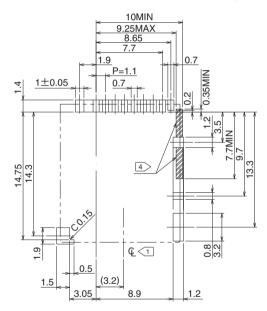
Note  $\bigcirc$  indicates the center line of the microSD card slot.
