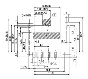
Q indicates the center line of the microSD card slot.
