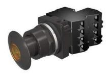
30mm BlackMax, Epoxy Coated Corrosion Resistant Complete Metal Unit Illuminated Push-Pull Operator Full Voltage, 120V AC/DC LED Lamp Mushroom Head Cap Small 1 3/4" (44.5 mm) Metal, Black with Amber Lens 3 Position Pull-Momentary/Push-Maintained 1 N.C.+1 N.C. Extra Late Break Heavy Duty Contacts, A600/P600 UL Listed, CSA Certified NEMA 1,3,3R,4,4X,12,13 & Automotive Standards
