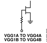
Figure 8. VGG1A to VGG4A and VGG1B to VGG4B Interface Schematic
