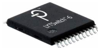
Figure 2. High Creepage, Safety-Compliant InSOP-24D Package.
