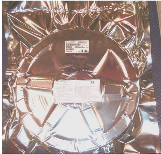
Fig. 2: Dry packed relay reel
