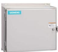
2-speed 3-phase motor starter Size 0 Two separate windings Constant horsepower Solid-state overload relays Low SPD OLR range 3-12A High SPD OLR range 3-12A 24VAC 50-60HZ coil Enclosure NEMA type 12 Dust/drip proof for indoors
