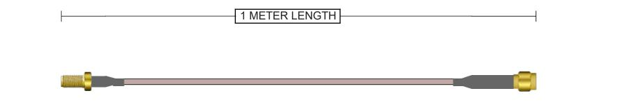
Connector A 132117 SMA Jack Straight Brass Gold + Heatshrink 50 Ohm RG-316 Continuity/Hi-Pot Connector B 132114RP SMA Plug Straight Brass Gold + Heatshrink
