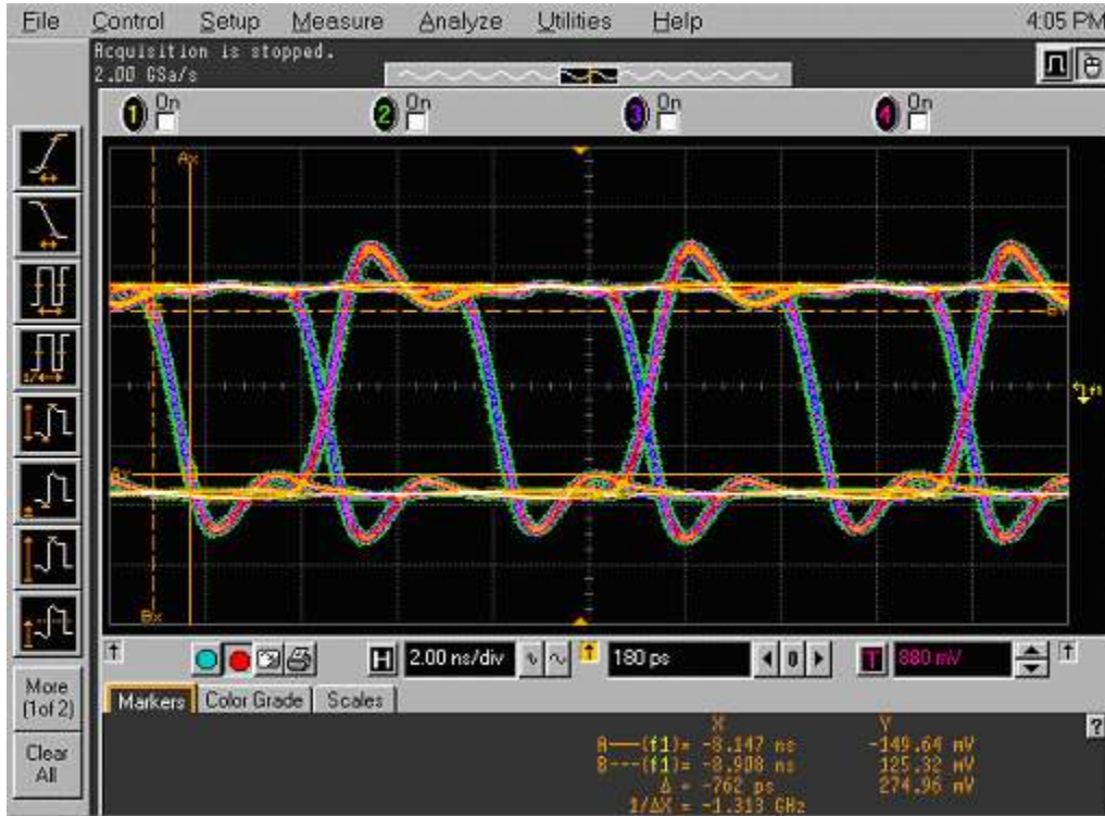
Figure 6 • LVDS Signal across RX Termination at 300 Mbps
