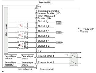
Non-voltage contact or NPN open-collector transistor
