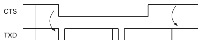
Figure 36-28: Transmitter Behavior when Operating with Hardware Handshaking
