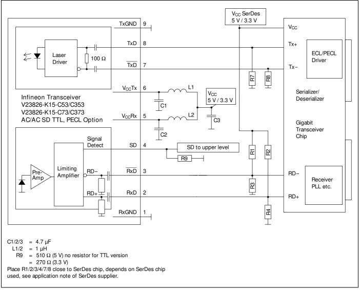
The power supply filtering is required for good EMI performance. Use short tracks from the inductor L1/L2 to the module  $V_{CC}Rx/V_{CC}Tx$ . We recommend a GND plane under the module for getting good EMI performance.
