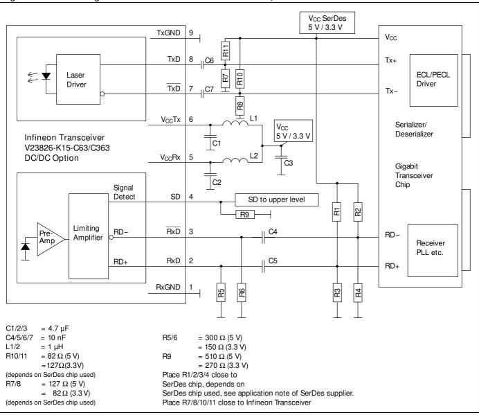
Values of R1/2/3/4 may vary as long as proper 50  $\Omega$  termination to V<sub>EE</sub> or 100  $\Omega$  differential is provided. The power supply filtering is required for good EMI performance. Use short tracks from the inductor L1/L2 to the module V<sub>CC</sub>RX/V<sub>CC</sub>TX. We recommend a GND plane under the module for getting good EMI performance.
