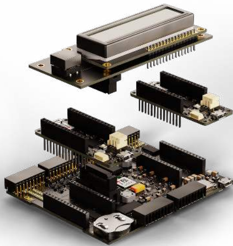
Example of a typical application for a solution including LCD Display and two Arduino MKR 1300 boards.
