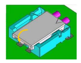
3. The reinforced lock is also released and the un-mating is complete
