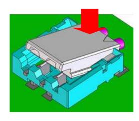
2. Pull up and release the simple lock
