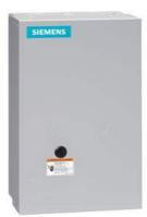
Non-reversing NEMA contactor, Size 3, Three phase full voltage, Contactor amp rating 90A, 3 wire (NO aux included), 24VDC coil, Non-combination type, Enclosure NEMA type 1, Indoor general purpose use, Standard width enclosure
