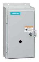
Non-reversing NEMA contactor, Size 2, Single phase full voltage, Contactor amprating 45A, 3 wire (NO aux included), 110V 50Hz / 120V 60Hz coil, Non-combination type, Enclosure NEMA type 12, Dust/drip proof for indoors, Standard width enclosure
