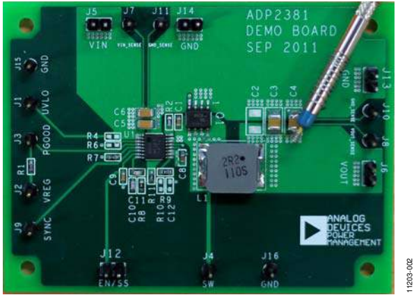
Figure 2. Measuring Output Voltage Ripple
