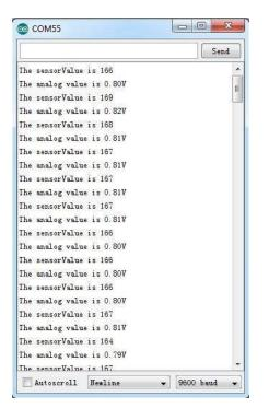
As default, Vref is generated by Arduino which is theoretically 5V. But actually that is a value afloat which results the deviation of the final data. This kind of inaccuracy is avoided when using Grove - I2C ADC, because it provides a strict 3.0V as Vref. To contrast, in the same condition, sensor values collected by the circuit with Grove - I2C ADC in the scope is shown below:
