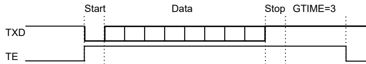
Figure 31-15. Example of TE Drive with Guard Time
