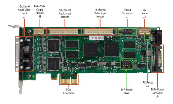
The card also supports sixteen channels of alarm I/O and an RS485 interface for remote camera control through an I/O header with an optional I/O card. Also a debug connector for UART and JTAG interfaces facilitate hardware and software debugging.
