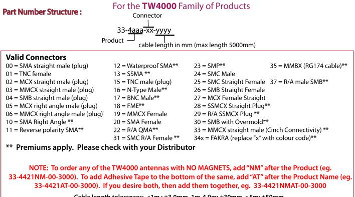
Cable length tolerances: <1m : ±3.0mm, 1m-4.9m: ±30mm, >5m: ±50mm
