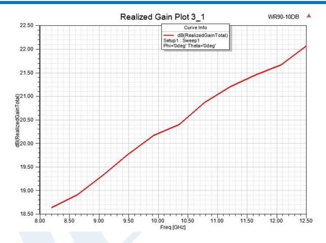
Click the following link (or enter part number in "SEARCH" on website) to obtain additional part information including price, inventory and certifications: WR-90 Standard Gain Horn with 20 dBi gain, End Launch SMA Female connector PEWAN090-20ELSF
