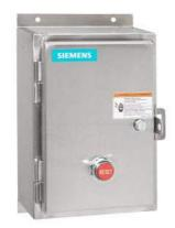
Non-reversing motor starter, Size 1, Three phase full voltage, Solid-state overload relay, OLR amp range 0.75-3.4A, Non-combination type, Encl. type 4X 304 S. Steel, Water/dust tight noncorrosive, Standard width enclosure
