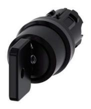
Key-operated switch O.M.R, 22 mm, round, plastic, lock number 73034, black, with 2 keys, 3 switch positions I-O<II, left latching, right momentary contact type, actuating angle 2x45°, 10:30h/12h/13:30h, key removal I, with laser labeling, inscription or symbol Customer-specific selection with SIRIUS ACT configurator (CIN)
