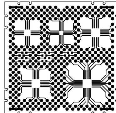
Supports 16 & 28 Pins with a .5mm pitch, 20 Pin with a .65mm pitch and
