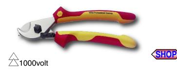
328 Cable Cutters. Insulation According to VDE 0682/part 201, Individually Tested. Drop-forged from durable CV steel, cutters additionally induction hardened, chrome & nickel plated, Mirror-polished. For copper and aluminum cables (not for steel wires), integrated release spring, one-hand locking, adjustable joint, anti-squeeze feature.
