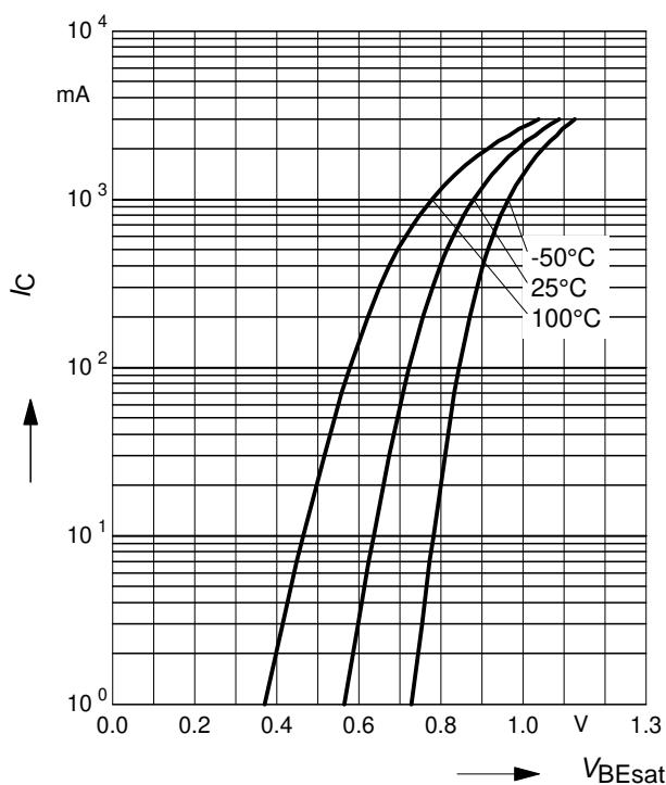
**Collector current**  $I_C = f(V_{BE})$
