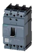
circuit breaker 3VA5 UL frame 125 breaking capacity class S 25kA @ 480 V 3-pole, line protection TM210, FTFM, In=90A overload protection Ir=90A fixed short-circuit protection Ii=10 x In UL489 SB (naval), 50 deg. cel. nut keeper kit on both sides
