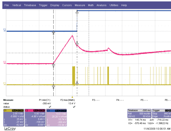
Figure 6. Start-Up Sequence Waveforms (Ch1 (Y), PFCDRV, Ch2 (R), V CCA , Ch3 (B), DUT V O )
