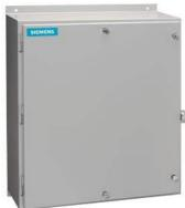
Non-reversing motor starter, Size 4, Three phase full voltage, Solid-state overload relay, OLR amp range 50-200A, 24VAC 50-60Hz coil, Non-combination type, Enclosure type 12, Dust/drip proof for indoors, Standard width enclosure
