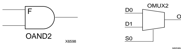
Figure 20: AND & MUX Symbols in XC4000X IOB
