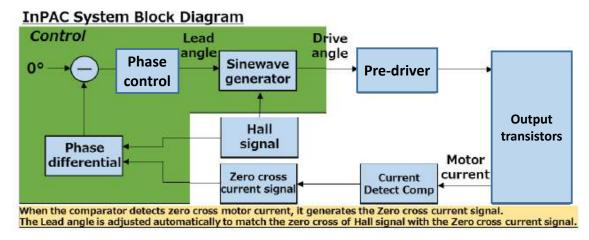
When the motor inductive voltage and the hall signal have a phase difference due to the mechanical shift of the hall sensor, the phase of the hall signal can be corrected in the range of -28.125° to 28.125° electrically by using the LA pin. Analog input of LA pin (Voltage range of 0 to 3.125 V is divided into 32.)
