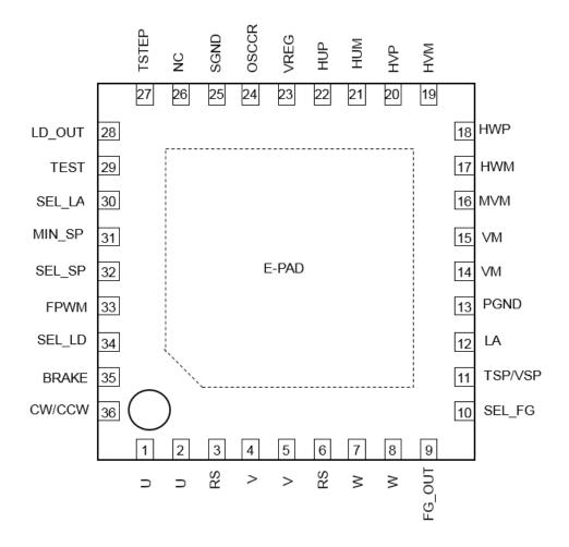
Note 1: Design the pattern in consideration of the heat design because the back side (E-PAD) have the role of heat radiation. The back side (E-PAD) should be connected to GND because it is connected to the back of the chip electrically.
