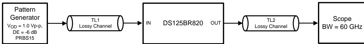
Figure 10. Test Setup Connections Diagram
