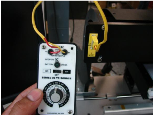
Image 48. TC connected to a TC socket
