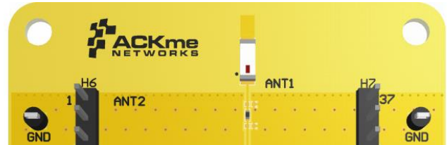
Figure 8 – Chip antenna layout example
