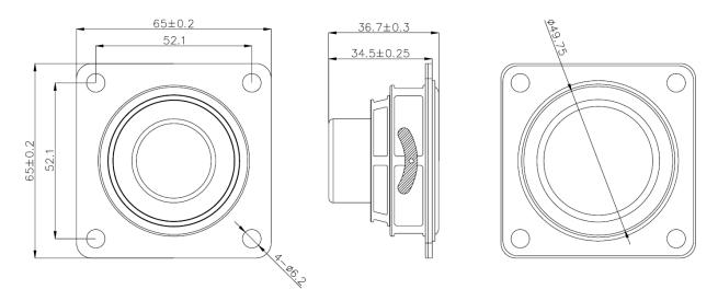
Note: Recommended speaker baffle opening is 53.6mm. Always test-fit prior to closing mechanical design. Please maintain at least 7mm distance between top of frame and next surface.
