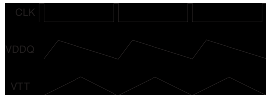
Figure 7. Optimal In-Phase Operation for DDR1
