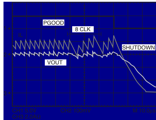
Figure 14. Over-Current Protection Waveforms
