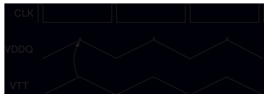
Figure 8. Noise-Susceptible In-Phase Operation for DDR2
