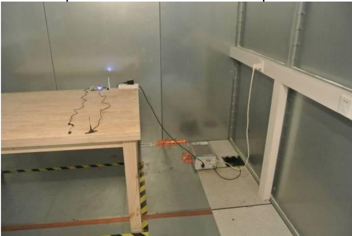
AC power line conducted emission Test Setup Photos
