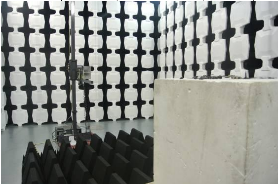
Description: Radiated Spurious Measurement Setup (Above 1GHz)
